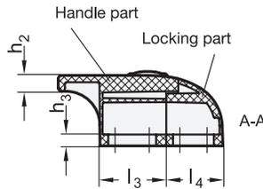
Assembly of handle part and locking part with hexagon head screw DIN 933-M6 or hexagon nut DIN 936-M6
