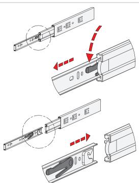
Type F has additionally a detach function through which the extension slides can be completely separated from one another in the area of the middle and inner slide. This feature not only facilitates mounting. It also allows the extension to be quickly removed, for example, when frequent maintenance work is performed on the components located behind.
