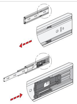
Telescopic slides GN 1414 have a dampened self-retracting mechanism, which is also called "soft-close". The dampened self-retracting mechanism is divided into two main functions and offers the best possible ease of use on closing the extension.
