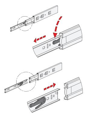
Type F has additionally a detach function through which the extension slides can be completely separated from one another in the area of the middle and inner slide. This feature not only facilitates mounting. It also allows the extension to be quickly removed, for example, when frequent maintenance work is performed on the components located behind.
