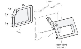
The installation recess in the door, cover or hatch for mounting the latch with gripping tray, must be cut as shown in the outline drawing.
